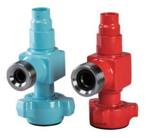
Aifuel pressure (safety) relief valves are a type of spring reset valves, which are designed to protect against overpressure from pump supply in the flow line. When the liquid pressure in the system exceeds the preset pressure of the pressure relief valve, the pressure relief valve is activated, and the fluid is discharged through the outlet to release the pressure;
