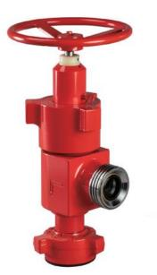
The chock valve adjusts the flow rate and pressure by adjusting the fluid flow in the manifold, and is mainly used for chock manifolds, flow manifolds and test manifolds. · The core component of Aifuel chock valve is forged by stainless steel with advaned erosion and abrasion resistant characteristics;
